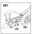
Insert the driveshaft into the clutch drum, then attach the gearbox to the shaft tube as aligning the positioning holes and fasten the screw (A). Fasten the clamp bolt (B) firmly. (SE1)
